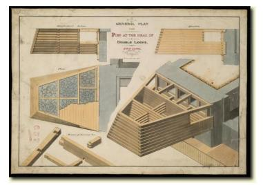
Figure 2. Pier plans drafted for the first enlargement of the Erie Canal. Plans such as this would have been unimaginable before the founding of the United States' first engineering schools and institutions.
