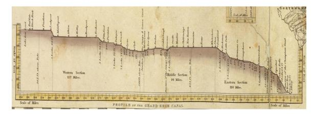
Figure 1. 1832 profile of the completed Erie Canal. The reasoning for beginning construction in the middle section is evident by its relatively small change in elevation compared to the western and eastern sections.
