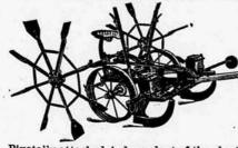
Pivotally attached, independent of the planter, allowing lateral flexibility,—the point that makes it successful.
