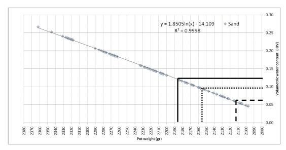
**Figure 3-1.** Relationship between pot weight and volumetric water content and of a sandy textured soil. Pot saturation (—PS), Pot capacity ("PC), Permanent wilting point (---PWP)
