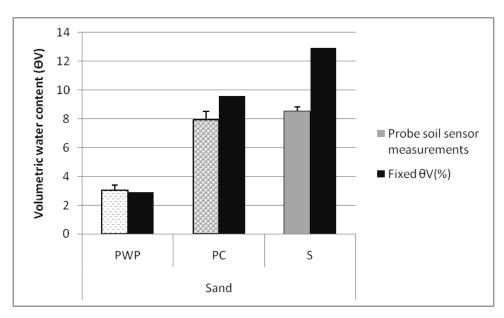
**Figure 3-2.** Evaluation of soil water content regimens by two methods in a sandy soil texture: manual weighing of pots (fixed  $\theta_V$ , %) and an electronic probe sensor. Probe soil sensor bars are the average of three replications.
