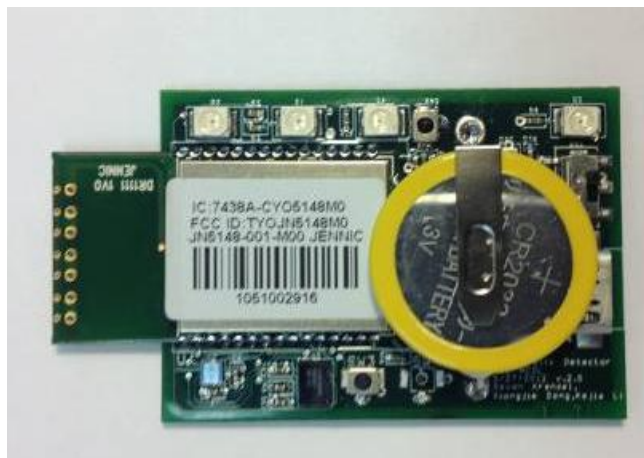
Figure 7.1 Custom accelerometer hardware.
