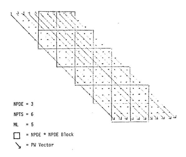
Figure 1: Block Tridiagonal Jacobian Matrix for PDE's and Its Storage in the PW Vector
