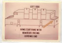
Question used in booklet for Method II. 13. Hang curtains with numbers facing \_\_\_\_\_ end. Answer to question No. 12. 10 11 Slide No. 14. Schematic of left side of dishwashing machine with arrows pointing to the location of hooks. Sign reading "Hang No. 10 and 11 curtains on hooks."
