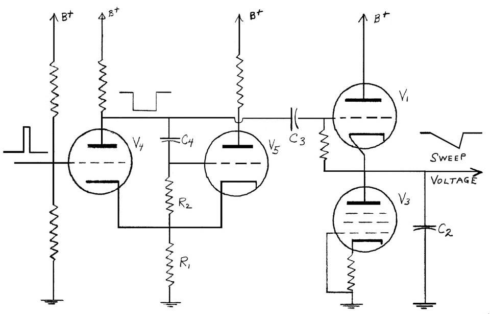
will develop a potential across cathode resistor  $R_1$  which will cause tube  $V_4$  to cut off.
