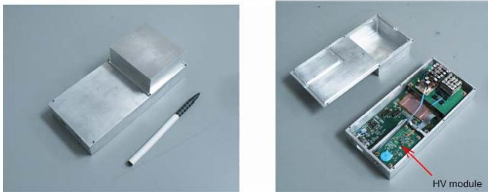
Figure 4.26: The two detector modules with the preamplifier board in a test box. Courtesy of Aleksey Bolotnikov at BNL.
