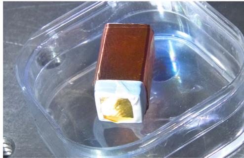
Figure 4.21: CdZnTe Frisch collar detector fabricated at S.M.A.R.T. laboratory at KSU. The picture is taken at Brookhaven National laboratory (BNL) after delivery of the devices.
