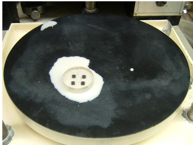
Figure 4.3: Polishing CdZnTe crystals on polishing pads
