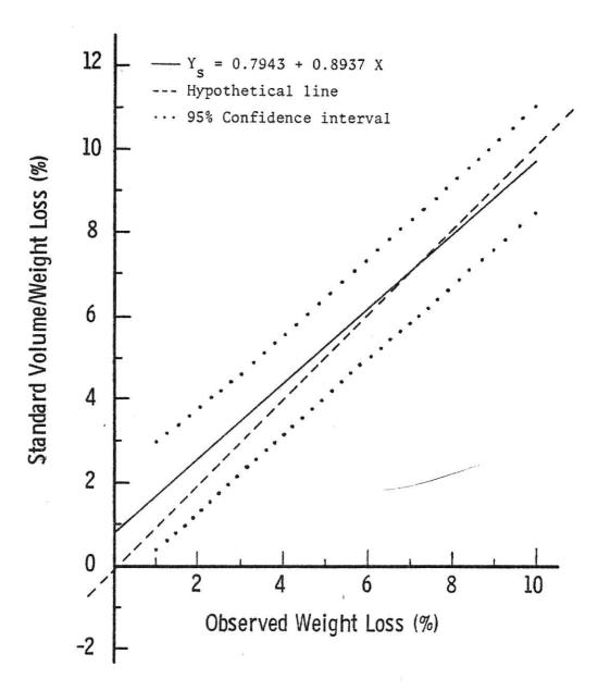
Figure 8. Relationship between percent weight loss estimated by the Standard Volume/Weight Method and the percent Observed Weight Loss produced in wheat by <u>Sitophilus zeamais</u> (Mots.) at 26 ± 2°C and 68 ± 5% r.h. R<sup>2</sup> = 0.9618.
