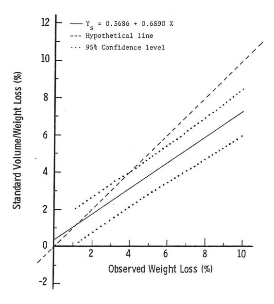
Figure 7. Relationship between percent weight loss estimated by the Standard Volume/Weigh Method and the percent Observed Weight Loss produced in sorghum by Sitophilus zeamais (Mots.) at  $26 \pm 2^{\circ}\text{C} \text{ and } 68 \pm 5\% \text{ r.h. } \text{R}^2 = 0.9668.$
