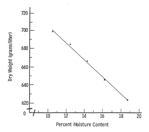
Figure D-5. Standard baseline curve for the experiment for dry weight of a liter of wheat.
