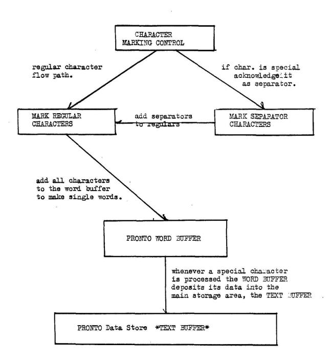
fig 3. PRE-PROCESSOR FLOW.
