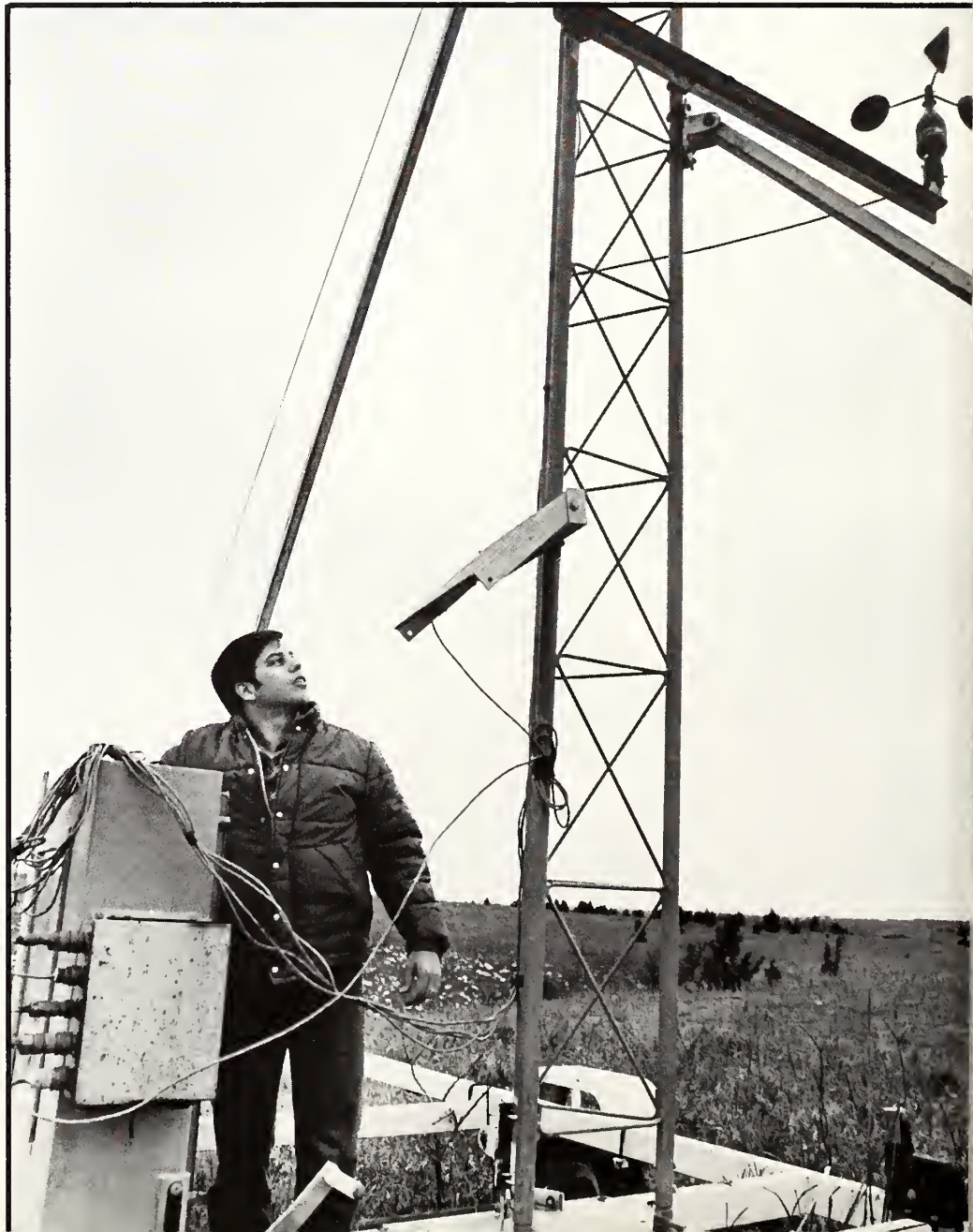
WIND POWER — John Gogolski, graduate in electrical engineering, inspects the wind velocity data gathering system which he designed. — Photo by Wes Wilmers
