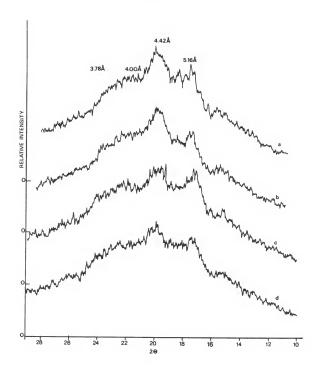
Fig. 13. X-Ray pattern of bread at day 14 storage (240C).
