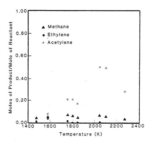
Fig. 3.16 Product yields as a function of temperature for the pyrolysis of 1.36 mol% benzene/ 0.07 mol% cyclohexane in argon with dwell times near 2.5 msec.
