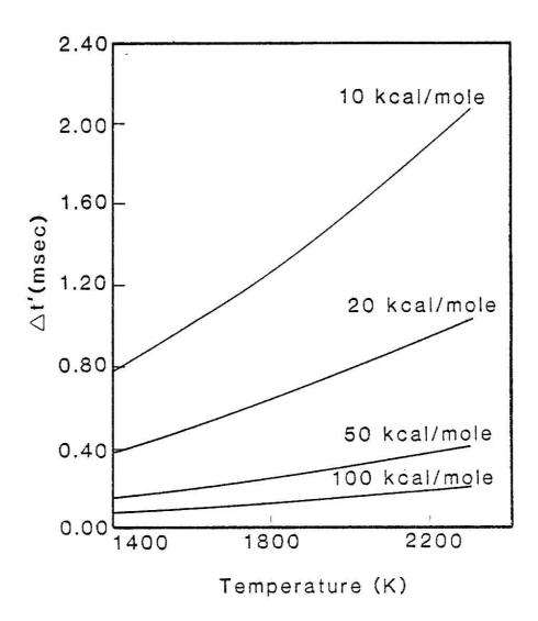
Fig. A.2 Finite cooling rate correction as a function of reaction temperature for specified activation energies
