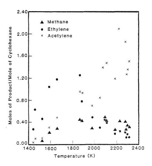
Fig. 3.3 Product yields from the pyrolysis of 1.3 mol% cyclohexane in argon as a function of reaction temperature for non soot runs with dwell times of 1.0-1.5 msec
