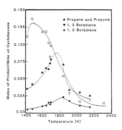
Fig. 3.7 Yields of  $C_3$  and  $C_4$  products as a function of reaction temperature for the pyrolysis of 1.3 mol% cyclohexane in argon with dwell times of 1.0-1.5 msec
