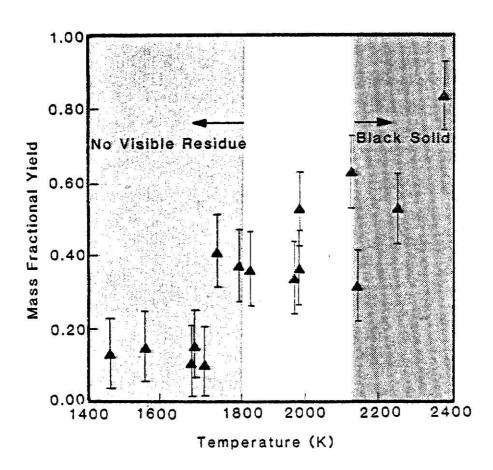
Fig. 3.19 Mass fractional yields of residue as a function of temperature for the pyrolysis of 1.3 mol% cyclohexane in argon with dwell times near 2.5 msec.
