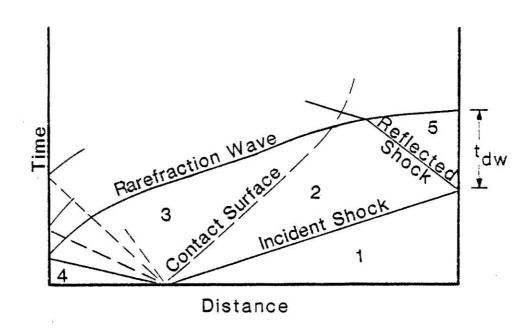
Fig. 2.1 A time versus distance diagram of the waves in a shock tube
