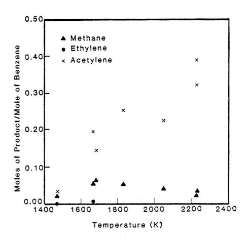
Fig. 3.10 Product yields as a function of temperature for the pyrolysis of benzene with dwell times near 2.5 msec.
