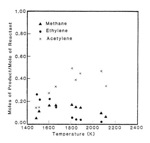
Fig. 3.18 Product yields as a function of temperature for the pyrolysis of 1.07 mol% benzene/ 0.36 mol% cyclohexane in argon with dwell times near 2.5 msec.
