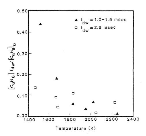
Fig. 3.8 Percent of benzene remaining after the pyrolysis of 1.3 mol% benzene in argon
