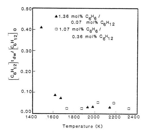
Fig. 3.11 Percent of cyclohexane remaining after pyrolysis of benzene/cyclohexane mixtures with dwell times of 1.0-1.5 msec.
