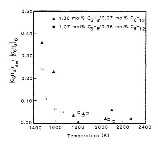
Fig. 3.14 Percent of benzene remaining as a function of reaction temperature for benzene/cyclohexane mixtures with dwell times near 2.5 msec.
