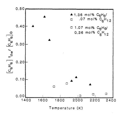
Fig. 3.13 Percent of benzene remaining as a function of reaction temperature for benzene/cyclohexane mixtures with dwell times of 1.0-1.5 msec.
