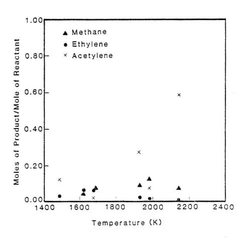
Fig. 3.15 Product yields as a function of temperature for the pyrolysis of 1.36 mol% benzene/ 0.07 mol% cyclohexane in argon with dwell times of 1.0-1.5 msec.
