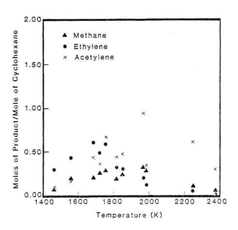
Fig. 3.6 Product yields as a function of temperature for the pyrolysis of 1.3 mol% cyclohexane in argon with dwell times near 2.5 msec and designated as soot runs
