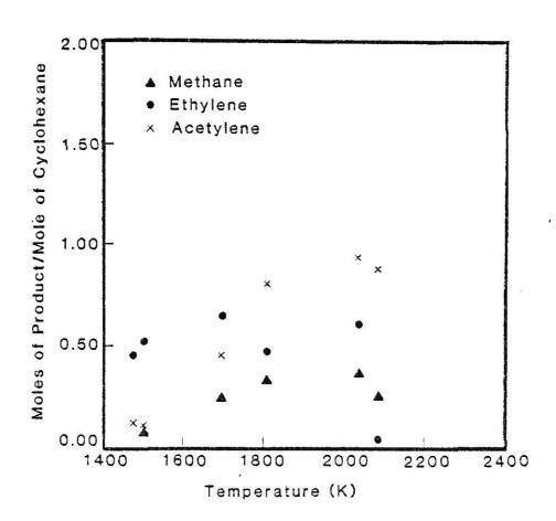
Fig. 3.4 Product yields as a function of temperature for the pyrolysis of 0.8 mol% cyclohexane in argon
