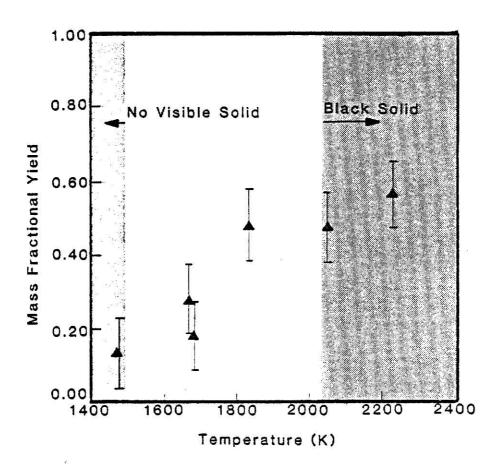
Fig. 3.20 Mass fractional yield of residue as a function of temperature for the pyrolysis of 1.3 mol% benzene in argon
