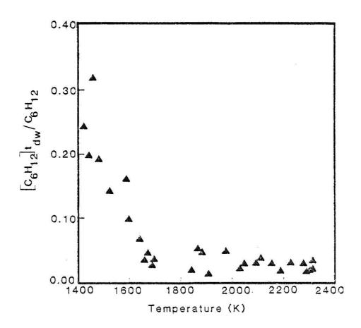
Fig. 3.1 Percent of cyclohexane remaining after pyrolysis of 1.3 mol% cyclohexane in argon as a function of reaction temperature for runs with dwell times of 1.0-1.5 usec (non soot runs)
