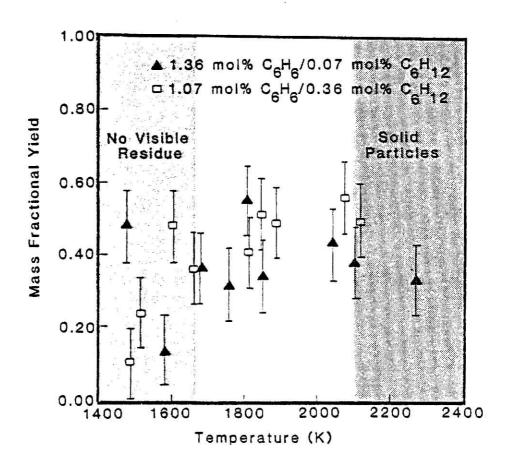
Fig. 3.21 Mass fractional yield of residue as a function of temperature for the pyrolysis of benzene/cyclohexane/argon mixtures
