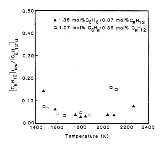
Fig. 3.12 Percent of cyclohexane remaining after pyrolysis of benzene/cyclohexane mixtures with dwell times near 2.5 msec.
