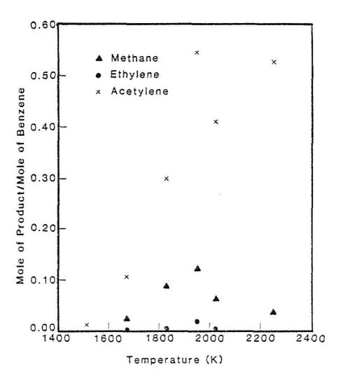
Fig. 3.9 Product yields as a function of temperature for the pyrolysis of benzene with dwell times of 1.0-1.5 msec
