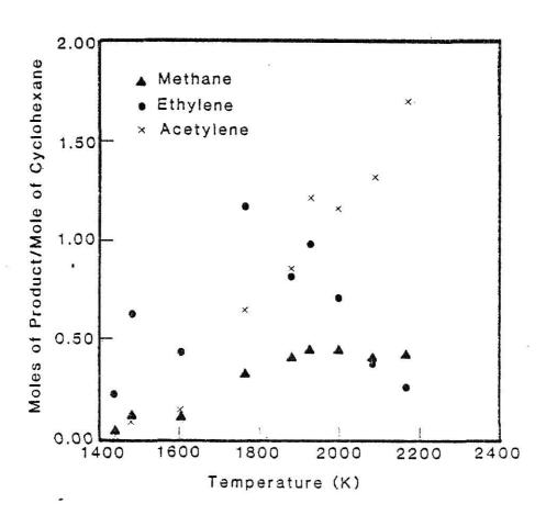
Fig. 3.5 Product yields from the pyrolysis of 1.3 mol% cyclohexane in argon with dwell times of 1.0-1.5 msec and designated as soot runs
