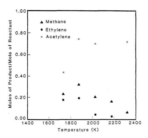
Fig. 3.17 Product yields as a function of temperature for the pyrolysis of 1.07 mol% benzene/
