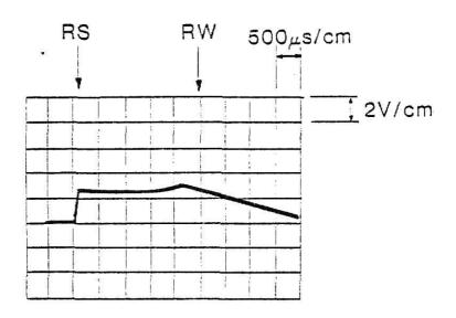
Fig. 2.4 Example of oscillogram of pressure history of gases in experimental section
