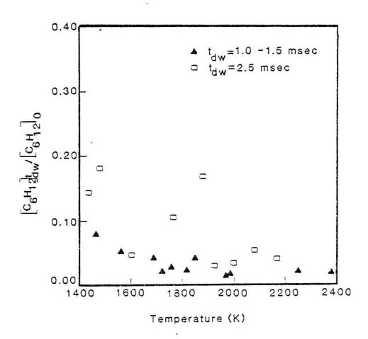
Fig. 3.2 Percent of cyclohexane remaining after pyrolysis of 1.3 mol% cyclohexane in argon as a function of reaction temperature for experiments designated as soot runs
