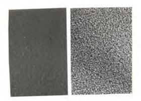
observed in the diffraction pattern of heat treated Co<sub>50</sub>Al<sub>50</sub> films indicate an ordered bcc- CoAl phase along with strong Co<sub>3</sub>Al reflections. The grain sizes of the former vary between 100 A and 200 A, while those of the latter range from 1000 A to 1100 A. The domain structure exhibits further coarsening and there is no specific orientation of the anisotropy components.
