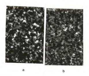
Figure 3.15 : Magnetic domain structure of as-deposited (a), and heat treated (b)  ${\rm Cos_0\,Al_{20}}$  thin films.
