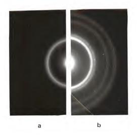
Figure 3.14 : Microstructure of as-deposited (a), and heat treated (b)  $\mathrm{Co}_{80}\,\mathrm{Al}_{20}$  thin films.
