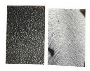
Figure 3.20 : The diffraction pattern, the microstructure, and the domain structure of as-deposited (a) and heat treated (b),  $Co_{50}Al_{50}$  thin films.
