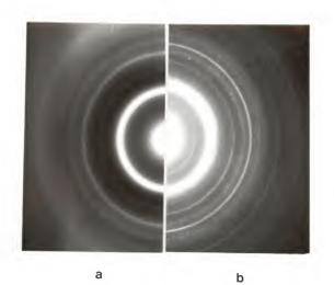
Figure 3.17 : Microstructure of as-deposited (a), and heat treated (b)  $\rm Co_{70}\,AI_{30}$  thin films.
