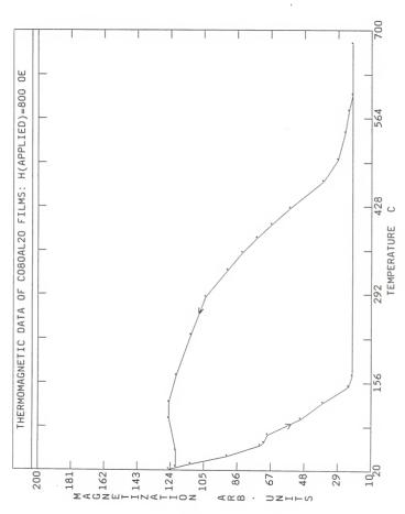
Figure 3.9 : Thermomagnetic data for  $\mathrm{Co}_{60}\mathrm{Al}_{40}$  thin films.
