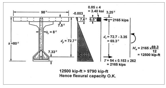
Figure C. 4 Calculation of the flexural strength at the mid-span
