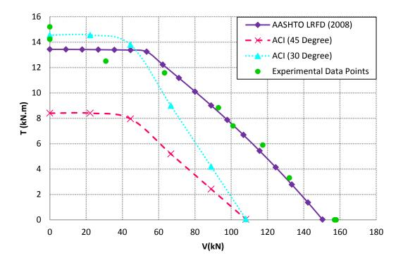
Figure A. 5 Shear-torsion interaction diagrams along with experimental data for specimens tested by Klus (1968)
