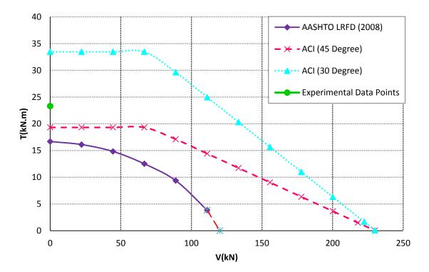
Figure 5.12 Shear-torsion interaction diagram for NU-2
