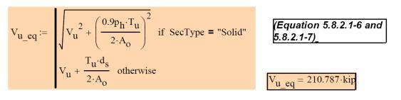
This equivalent V<sub>u\_eq</sub> is just for checking the adequecy of the section, when needed, otherwise the shear and torsional steel need to be evaluated as needed and then added up (shear as per 5.8.3.3 and Torsion as per 5.8.3.6.2)
