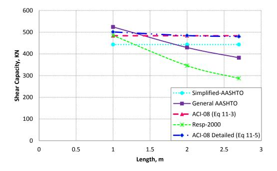
Figure 5.1 Predicted shear strength along the length of BM100, normal strength, non-prestressed simply supported reinforced concrete beam
