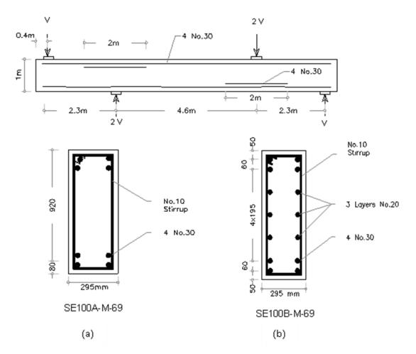
Figure 2.4 (a) Cross-section of high-strength, continuous non-prestressed reinforced concrete beam (b) Cross-section with the crack control (skin) reinforcement.
