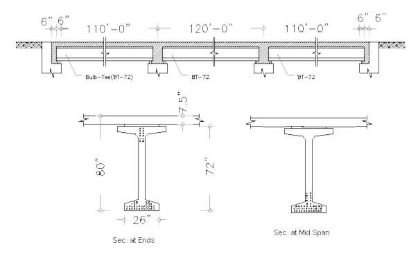
Figure 2.6 Profile and sections at mid-span and at end of high strength, continuous Bulb-T (BT-72) member
