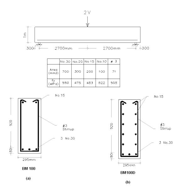
Figure 2.3 (a) Cross-section of normal strength, non-prestressed simply supported reinforced concrete beam (b) Cross-section with the crack control (skin) reinforcement.
