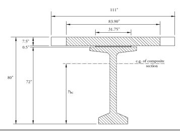
\*Note: If modulus of Elasticity for topping, slab, is different than modulus of elasticity for girder, determin **n=E<sub>c,slab</sub>/E<sub>c,beam</sub>** called modular ratio and multiply it by the area of slab( b<sub>eff</sub> x slab thickness). Add the given value to Area of Girder for total area of composite section.
