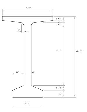
Figure A. 2 Cross-section (BT-72)
