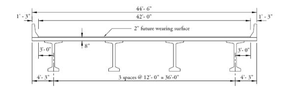
Figure A. 1 profile and section of the bridge girder (BT-72)
