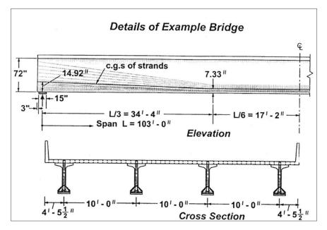
Figure C. 1 the girder used in this example, and a cross section of the bridge
