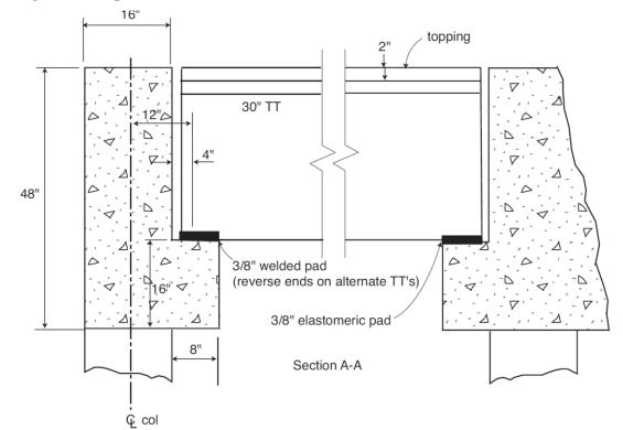
Figure C. 7 Spandrel beam cross section
