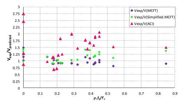
Figure 2.2 The ratio of experimental to predicted shear strengths Vs transverse reinforcement for the panels
