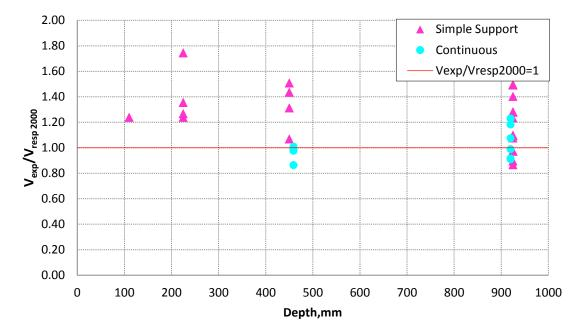
Figure 3.2 (Vexp/VResp-2000-Depth) Relationship for 34 reinforced concrete sections
