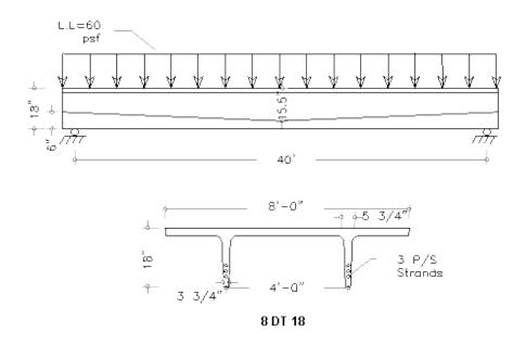
Figure 2.5 Profile and cross-section at mid-span of normal strength, simply supported, Double-T (8DT18) pre-stressed concrete member
