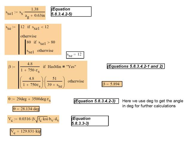
Designing the transverse reinforcement for <u>SHEAR</u> (Note that the  $A_v/s$  will be evaluated. Then when we have Torsion as well, we can add them appropriately depending on the type of section)
