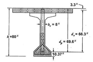
Figure C. 5 Calculating the section properties at 0.2L
