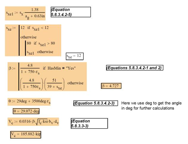
Designing the transverse reinforcement for <u>SHEAR</u> (Note that the  $A_v/s$  will be evaluated. Then when we have Torsion as well, we can add them appropriately depending on the type of section)
