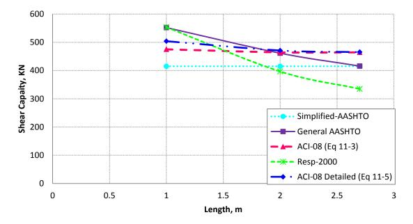
Figure 5.5 Predicted shear strength along the length of BM100-D, normal strength simply supported non-prestressed reinforced concrete beam with longitudinal crack control reinforcement
