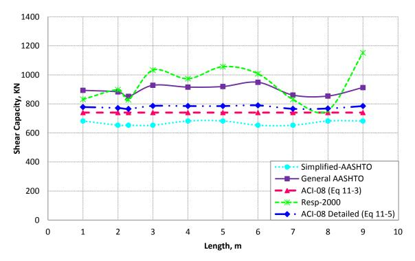
Figure 5.6 Predicted shear strength along the length of SE100B-M-69, high strength continuous non-prestressed reinforced concrete member with longitudinal crack control reinforcement
