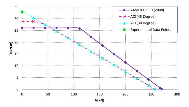
Figure 5.11 Shear-torsion Interaction diagram for High-Strength box section HU-3
