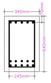
Figure 2.8 Typical beam section for RC2 series tested by Rahal and Collins (2003)
