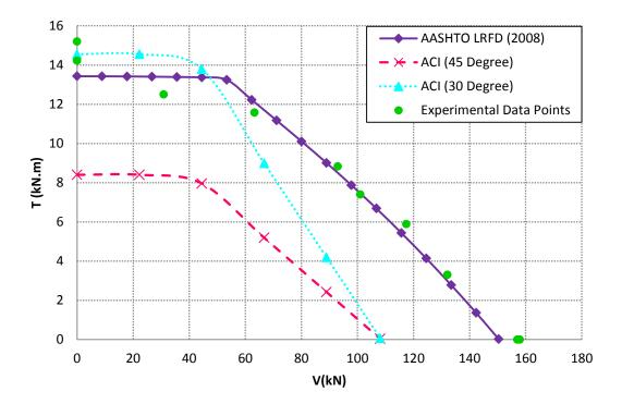
Figure 5.7 Shear-torsion interaction diagrams along with experimental data for specimens tested by Klus (1968)
