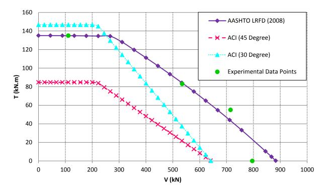
Figure 5.8 Shear-torsion interaction diagrams for RC2 series
