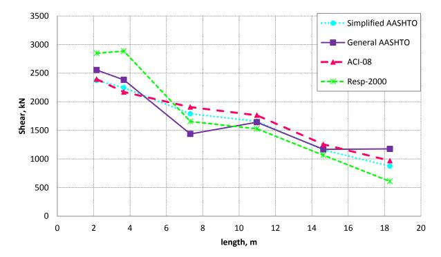
Figure 5.3 Predicted shear strength for Bulb-T (BT-72), high strength continuous pre-stressed concrete member
