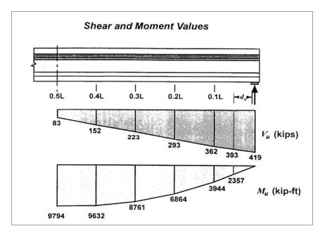
Figure C. 3 Demanded shear and moment values at various locations along the beam
