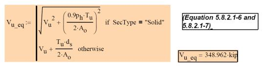
This equivalent V<sub>u\_eq</sub> is just for checking the adequecy of the section, when needed, otherwise the shear and torsional steel need to be evaluated as needed and then added up (shear as per 5.8.3.3 and Torsion as per 5.8.3.6.2)
