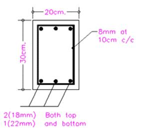
Figure 2.7 Typical beam section tested by Klus (1968)
