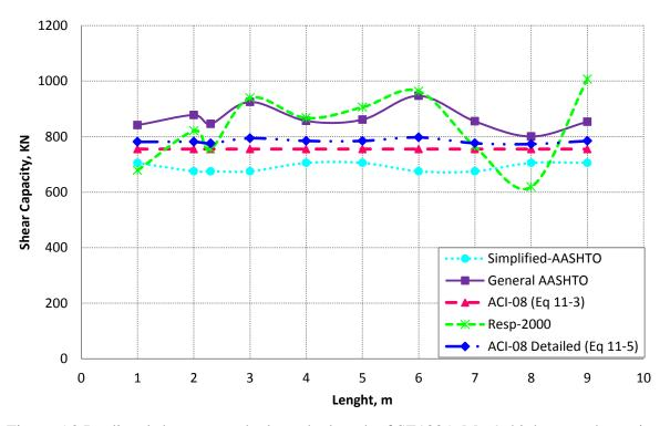
Figure 5.2 Predicted shear strength along the length of SE100A-M-69, high strength continuous non-prestressed reinforced concrete beam
