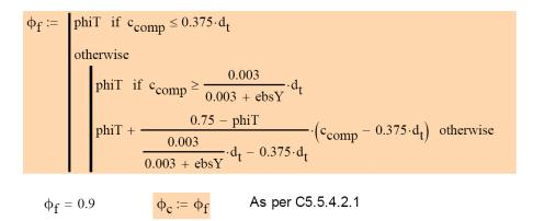
Evaluation of the shear and torsional strength reduction factors based on 5.5.4.2
