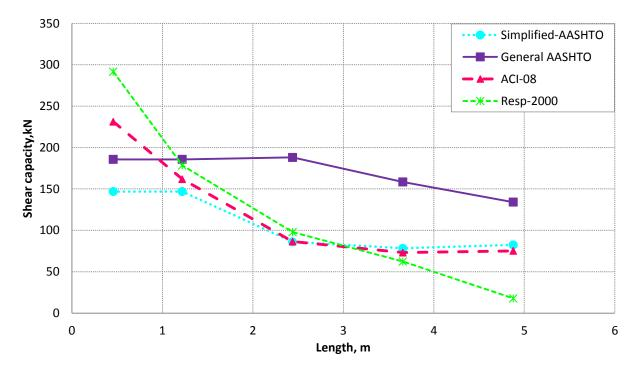
Figure 5.4 Predicted shear strength along the length of Double-T (8DT18), normal strength simply supported pre-stressed reinforced concrete beam
