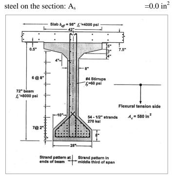
Figure C. 2 Beam cross section showing general geometry and reinforcement
