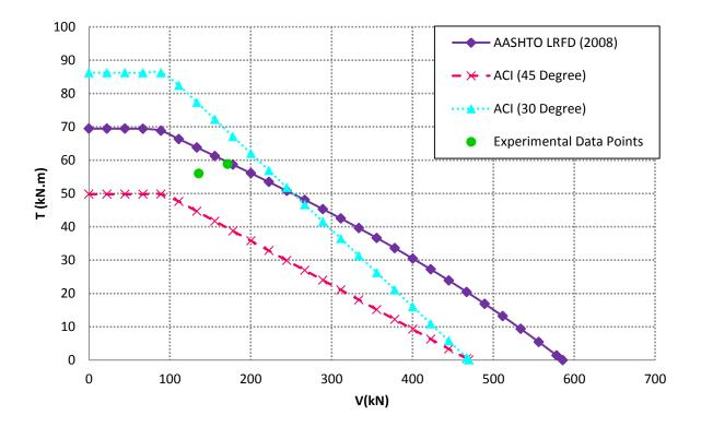
Figure 5.9 Shear-torsion interaction diagrams for High-Strength over-reinforced specimens HO-1, and HO-2
