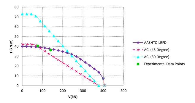
Figure 5.10 Shear-torsion interaction diagram for NO-1 and NO-2
