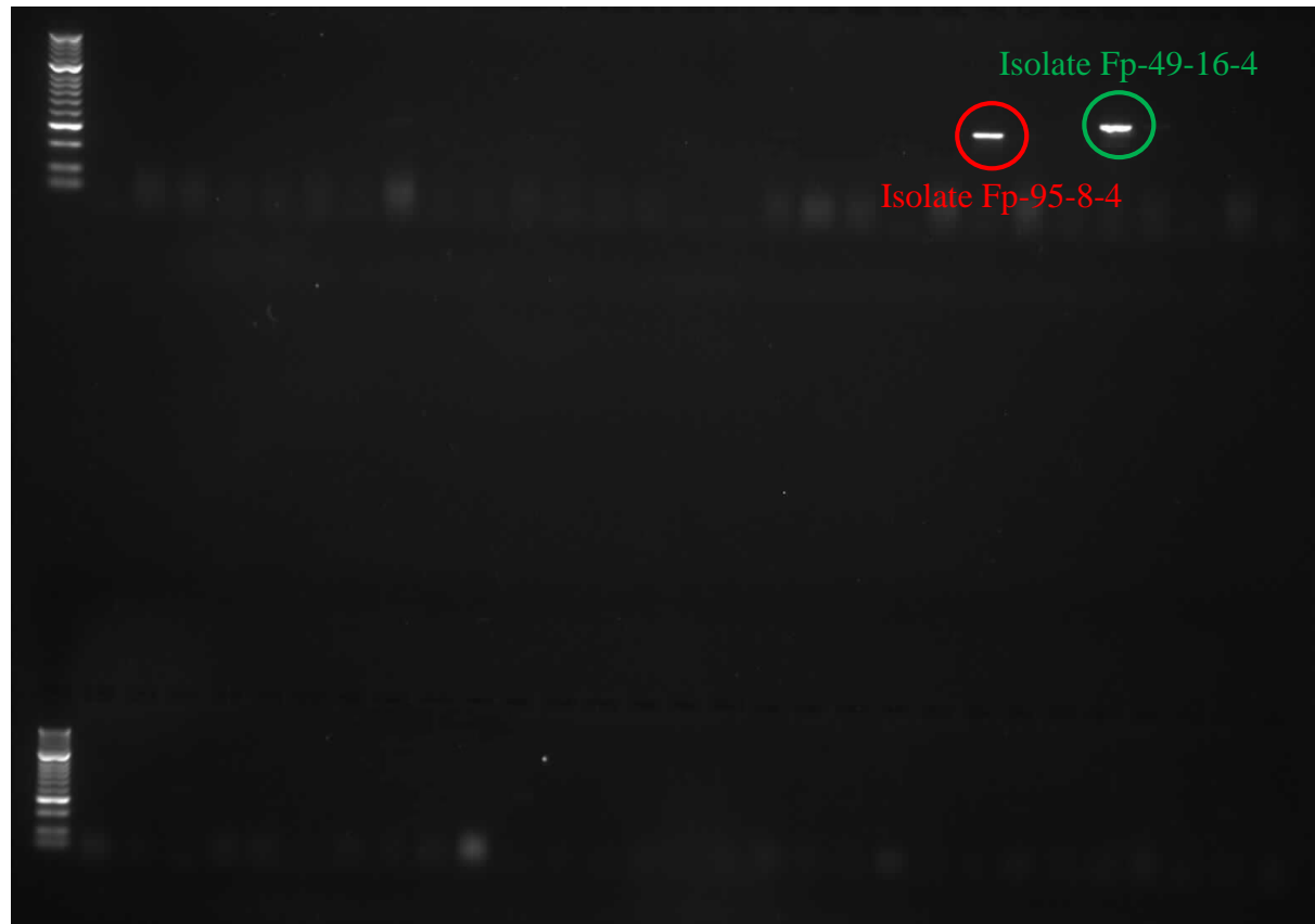
Figure 5.3 Multiplex end-point PCR assay using strain-specific primers for isolates Fp-49-16-4 and Fp-95-8-4 in 58 different F. proliferatum isolates showed specificity of the primers. Fp-49-16-4 had a 498bp amplicon and Fp-95-8-4 had a 454bp amplicon. 60 additional F. proliferatum isolates were tested in the exclusivity panels.
