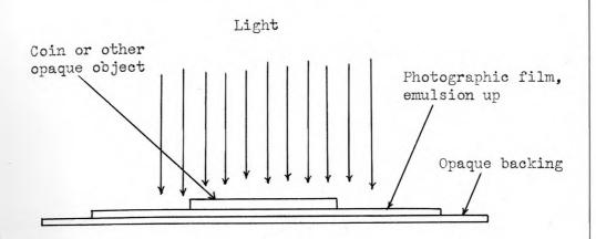
Fig. 1. Showing position of materials used in conducting experiments.
