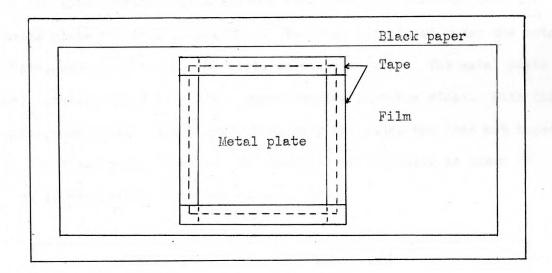
Fig. 13. Showing position of materials used in investigation of light path.
