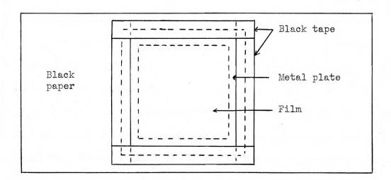
Fig. 8. Showing position of materials used for pressure and electronic transmission investigation.
