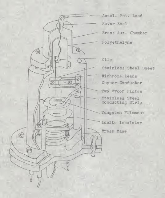
The only disadvantage to this source was the 20-minute operation of opening and resealing the three vacuum seals connecting the auxiliary chamber to the source chamber and the source chamber to the instrument and to a diffusion pump. The advantages were rigidity of source, less distortion of the filament, and a simpler removal of the filament leads for insertion of another sample.
