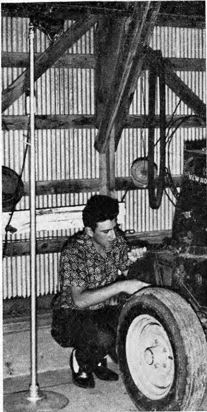
Gary Sallans, Herndon Cardinals Club in Rawlins county, made this portable shop light extra high so it would provide good light under all sorts of working conditions and on all sorts of equipment.
