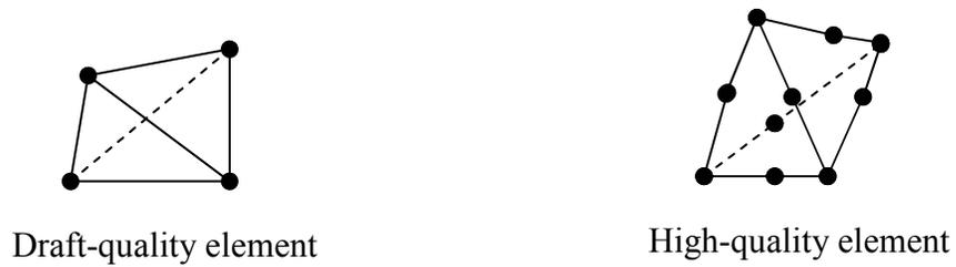
**Figure 3.3 Draft-Quality and High-Quality Solid Element (after SolidWorks, 2009)**
