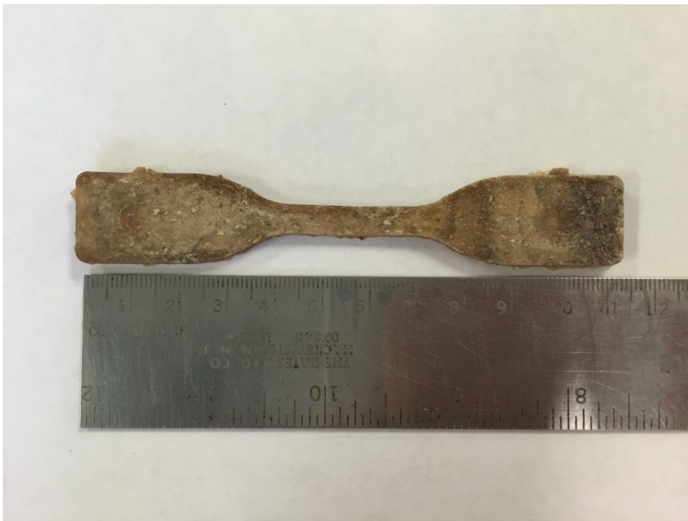
Figure 3.2 Injection molded bar from pilot-scale production of dental treats. Ruler for scale.
