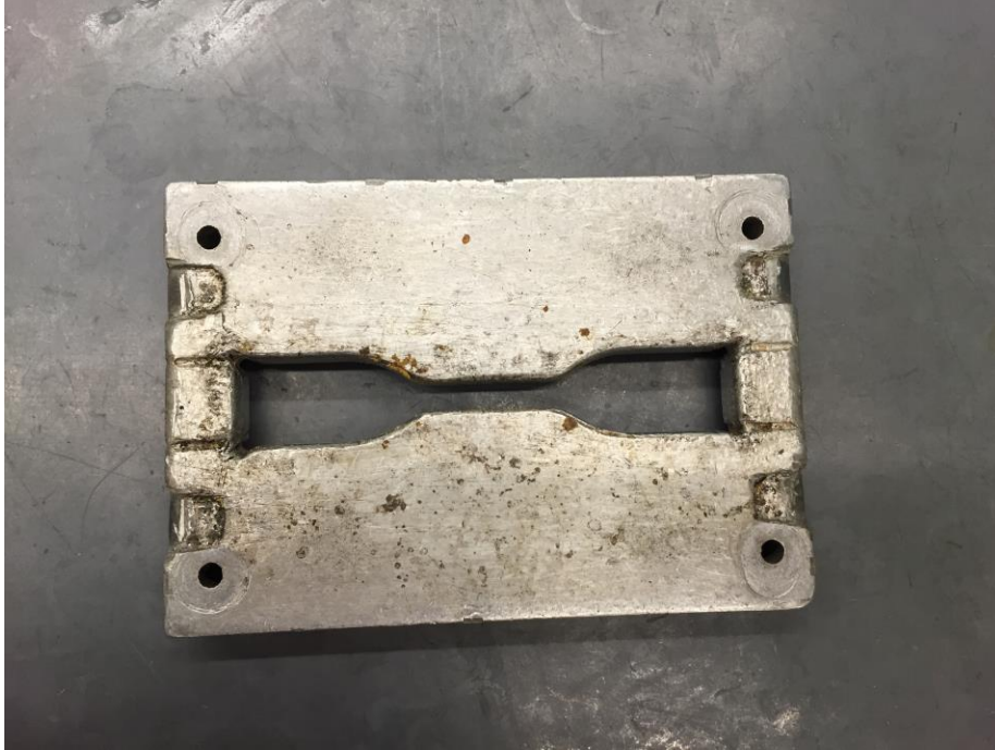
Figure 3.1 Mold used to create compression molded treats using a simplified formula of varying levels of low-bloom gelatin, gluten, and glycerin.
