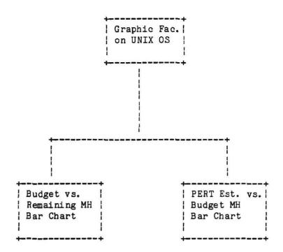
Figure 3-5. Hierarchy Block Diagram of Graphic Generation Software Component
