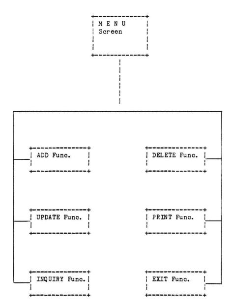
Figure 3-4. Hierarchy Block Diagram of Interactive Processing Software Component
