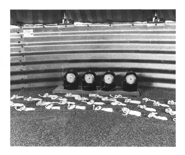
temperature readings were taken between 1000 and 1400 hours using a Hot Spot® portable potentiometer, model PP-62 (Fig. 3). Maximum and minimum daily outdoor temperatures for Manhattan, Kansas, recorded by the Kansas State University Physics Department, were obtained from U. S. Department of Commerce reports (Anonymous 1965-1974). The accuracy of all temperature measurements was  $\frac{1}{2}$  1°C.
