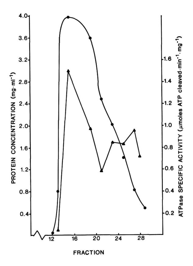
Fig. 4. DEAE (diethylaminoethyl) cellulose chromatography of myosin. The column (2.5 cm X 16 cm) was eluted at 32 ml per hour and 5 ml fractions collected. Protein concentration profile ( \_\_\_\_\_\_\_). ATPase specific activity profile ( \_\_\_\_\_\_\_\_).
