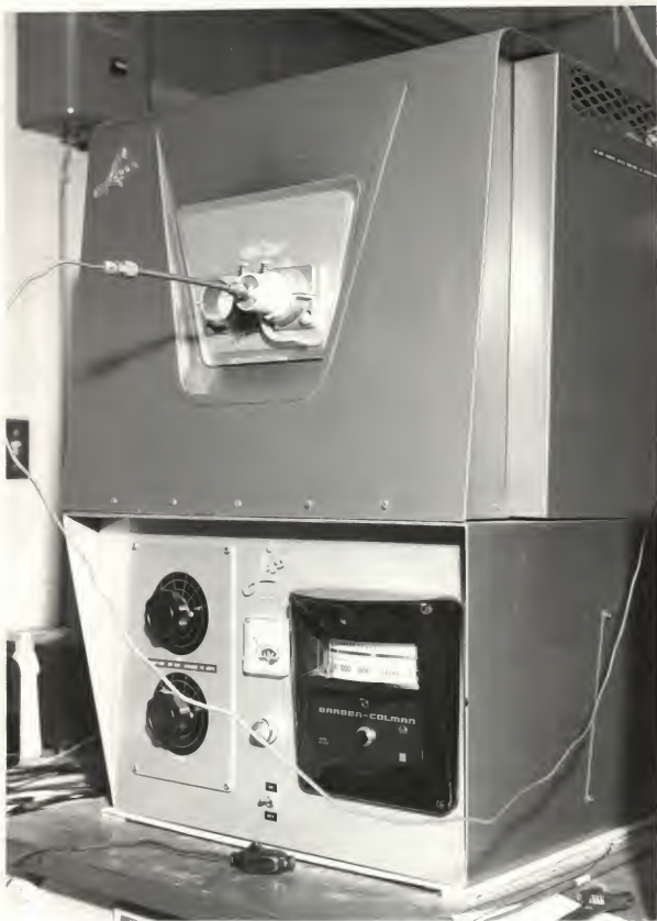
Fig. 7. A view of the LECO model 540 resistance furnace.
