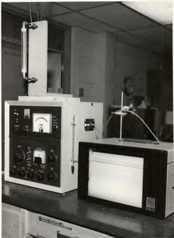
Fig. 8. A view of the 90P3 gas chromatograph and model 30 strip chart recorder.
