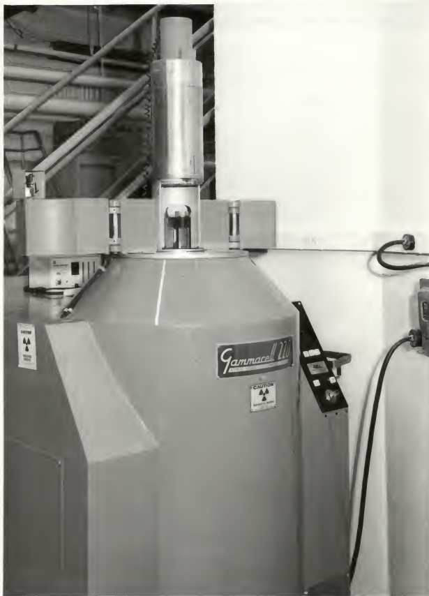
Fig. 6. External view of "Gammacell"-220 with a sample in the elevated irradiation chamber.
