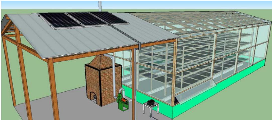
Figure 1: Schematic diagram of the biomass hybrid solar dryer set up in Ejura, Ghana.
