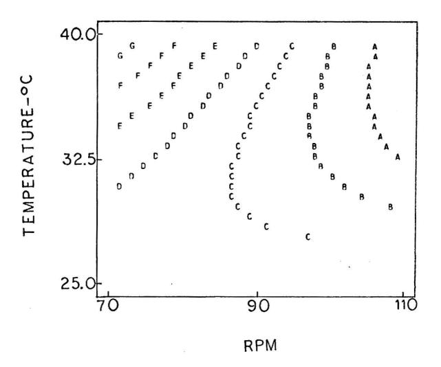
Fig. 4. Standard 'C' Flour. Contour plot of mixing time  $(C=3,\ D=3.5,\ E=4,\ F=4.5,\ G=5,\ H=5.5,$   $J=6,\ K=6.5,\ L=7,\ M=7.5,\ N=8,\ O=8.5,$   $P=9.0) \ \text{for rpm and temperature with absorption}$  held constant at 62.5% (optimum at 90 rpm and 25°C).
