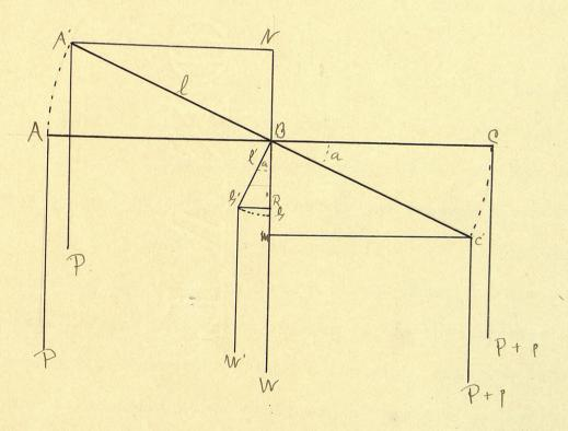
When the center of gravity is above the point B, the equilibrium of the balance is unstable and a slight addition of weight to either pan would cause it to turn upside down. Should the center of gravity be at B, the equilibrium would be indifferent and the beam would remain at rest in any position. Therefore the center of
