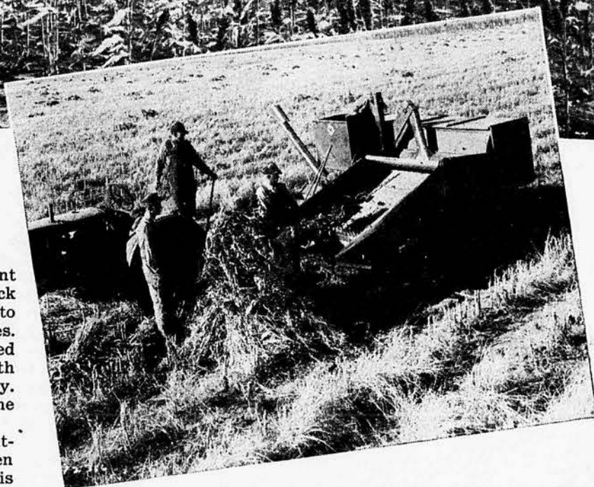
Combining from the shock, as shown here, is one of the popular methods of harvesting sorghum in Eastern Kansas. This outfit, owned by George Britting, Butler county farmer, is at work on the farm of Earl Mackey. This 5-foot machine threshes the grain as rapidly as 3 men can feed it.
