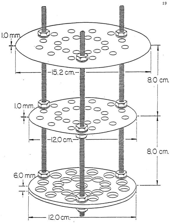
Figure 3. A Draft of a Plunger of the Bean Cooker Which Yields a Continuous Cookability Curve.
