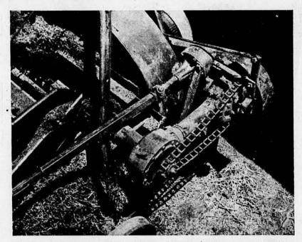
This closeup of the remodeled section on the blower shows how W. J. Brose added a stub gear and transmission that is connected to a drum shaft on their trailers to do the unloading.
