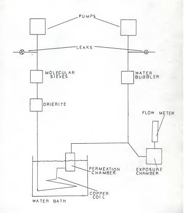
Figure 6: Calibration of the Permeation Tube
