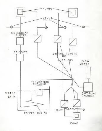
Figure 8: Permeation Chamber Containing Permeation Tube
