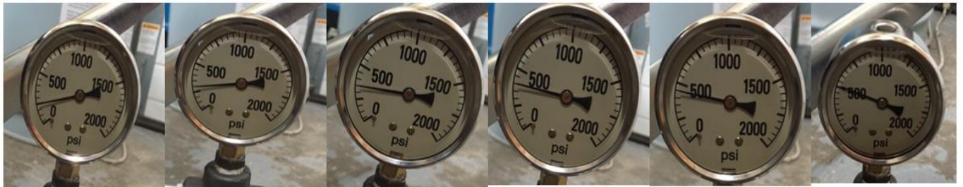
Figure 2.17 The pressure of each stage of the hydraulic test
