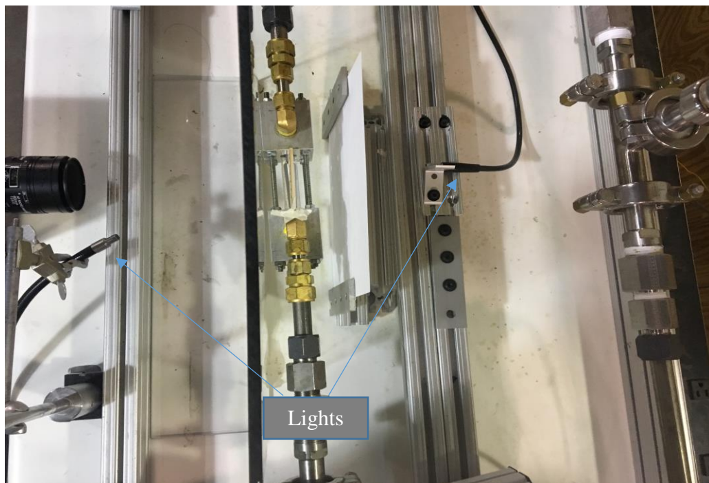
Figure 2.22 The top view of the test section to illustrate the lighting setup
