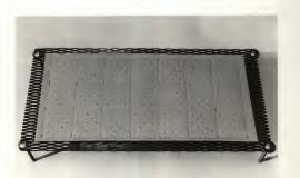
more mass, of course, required more oven heat to warm them to oven temperature and thus the bottom of the cracker stayed cool longer. The heat transfer problem was more pronounced with heavier racks. It appeared that mass of the baking surface had to be balanced with the weight of the cracker piece to obtain the desired baked product.
