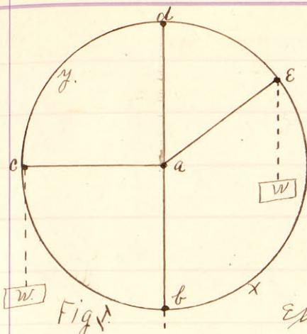
For a diagrammatic example of a uniformly loaded crank, let  $xy$  in Fig. I be the path of the crank and  $w$  the load to be lifted.
