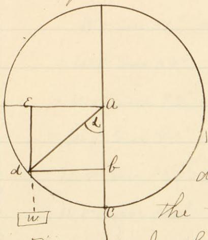
In Fig. III let ac represent a crank centred at a and loaded with a load w. Let  $\alpha$  equal the angle of rotation from the lower radius; ae the perpendicular distance from the point of rotation, a, to the line ed in the direction of the force.
