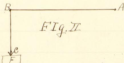
In Fig. II let  $A.B$ , called the lever arm, be the perpendicular distance from  $a$ , the point of rotation, to  $bc$  the line in the direction of the acting force  $F$ . Then M the moment equals  $F \times ab$ .
