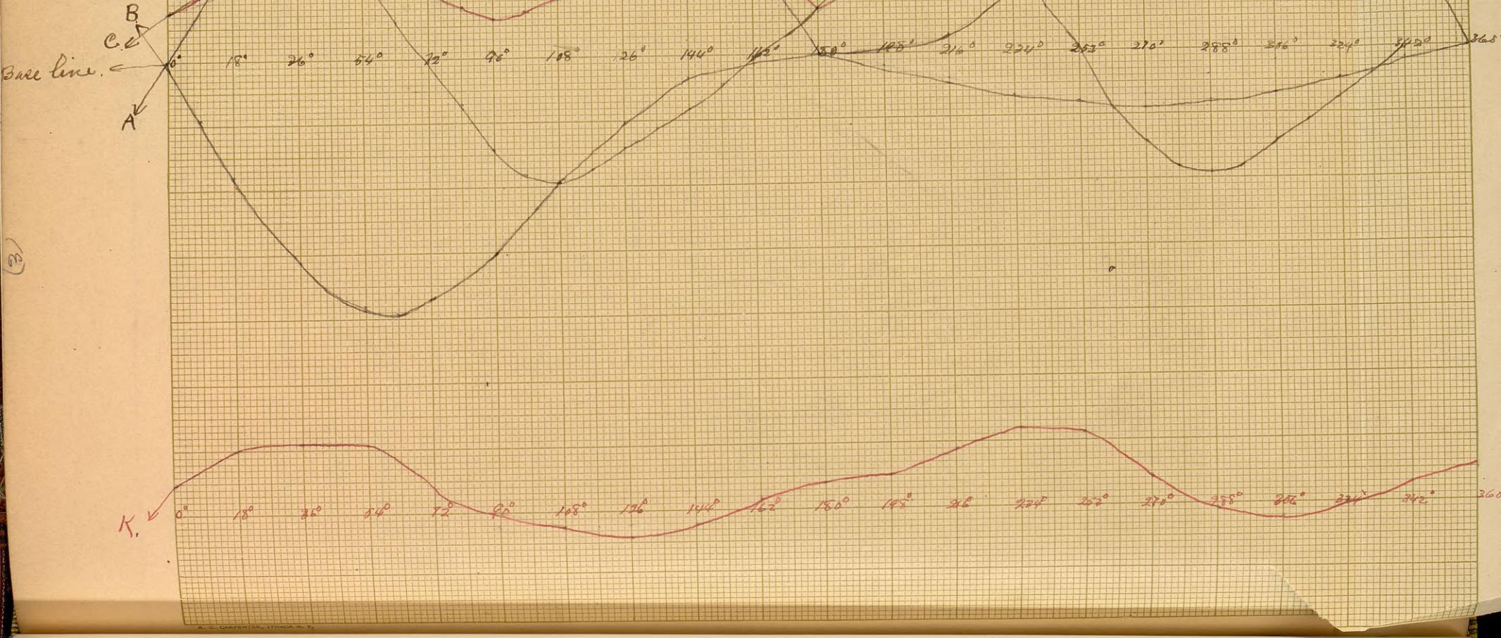
loaded crank. The results are shown on the plot page 3. The distances above the base line of the plot, represent the moments at various places, those along the base line represent the angles along the cranks path. The lines connecting these various points determine the moments of all the various positions of the crank in its rotation.
