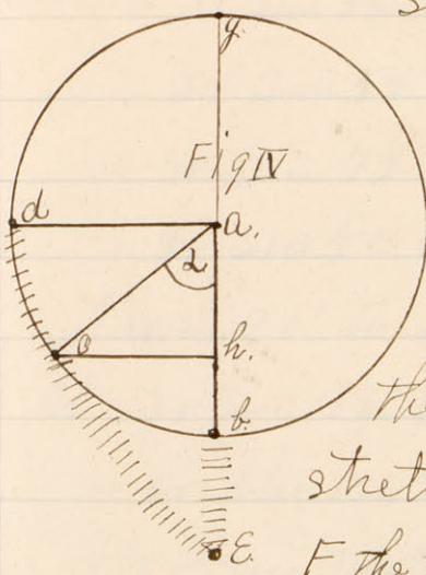
Suppose a spring as shown in Fig IV be fastened at the point c and attached to the crank ab. Let b = the tension of the spring when stretched from b to g, let z = the angle of rotation. Then the stretch of the spring at c, which is bh is to the stretch at e, which is be, as bh is to be.
