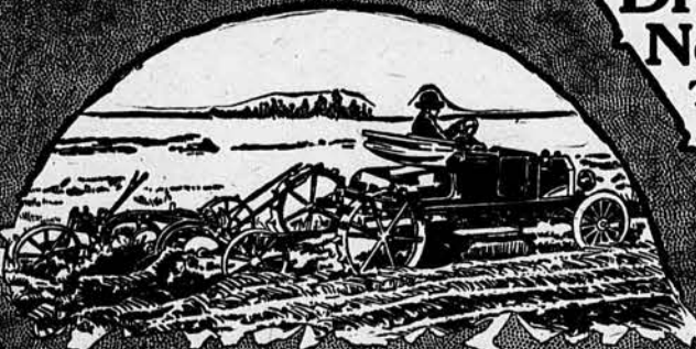
Breaking virgin sod, 7 in. deep with 2 bottom, 28 in. gang. (Reproduction from moving picture film.)
