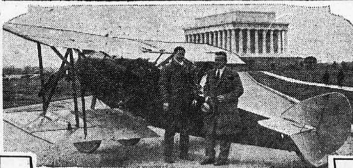
Lawrence Sperry Arrives in Washington With His Sport Messenger Airplane; He Flew From Garden City, Long Island, N. Y., to the Capital in Record Time; This Airplane has a Span of 21 Feet Across the Wings and Measures 20 Feet and 6 Inches From Nose to Tail; It is 17 Feet in Height and is Very Easy to Guide and Manipulate.
