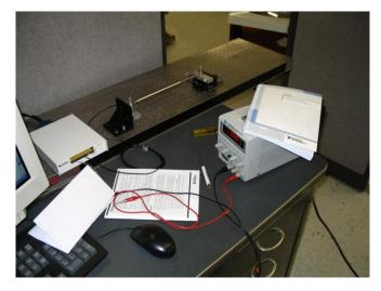
Figure C-15: LVDT Calibration Test
