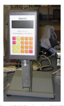
Figure B-1: Brookfield Engineering DV-III Rheometer
