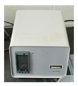
Figure B-6: Peltier Thermal Regulator PTR-1
