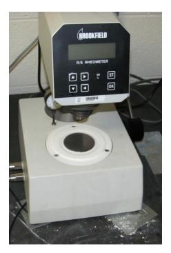
Figure B-4: Brookfield R/S-CPS Rheometer
