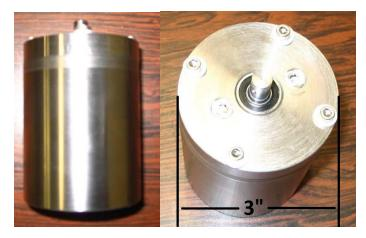
Figure 3-2: Viscous Latch
