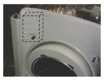
Figure 1-4: Dryer Door Latch Space Limitations
