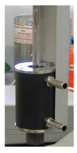
(A) SC4-28 Spindle (B) Temperature Control
