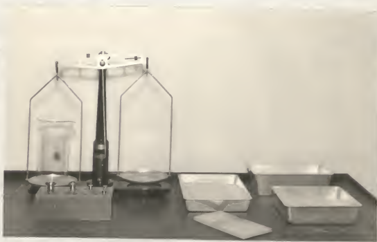
Fig. 4. Three pan sizes used, sand-weighing apparatus and sand-leveling board.
