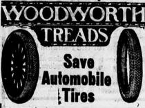
They are tire protectors, made of chrome leather studded with steel studs held on the tires by spring wires on each side. Anyone can easily fit them to any make of tires.
