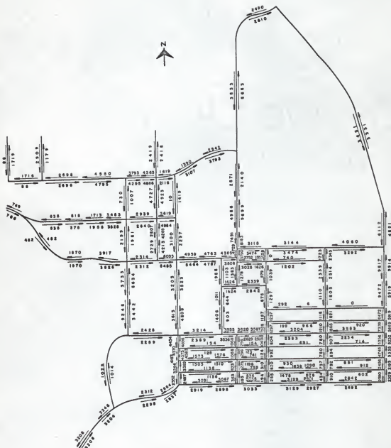
Fig.10. Average daily traffic volumes assigned to the major street network by the maximum principle method (Case 1).
