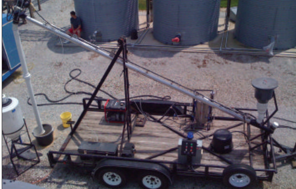
The continuous-ozonation flow system consists of applying high concentrations of ozone through a modified screw conveyor in the same flow direction of the grain going into a bin. Photo supplied by Carlos Campabadal and Lynntech, College Station, TX.
