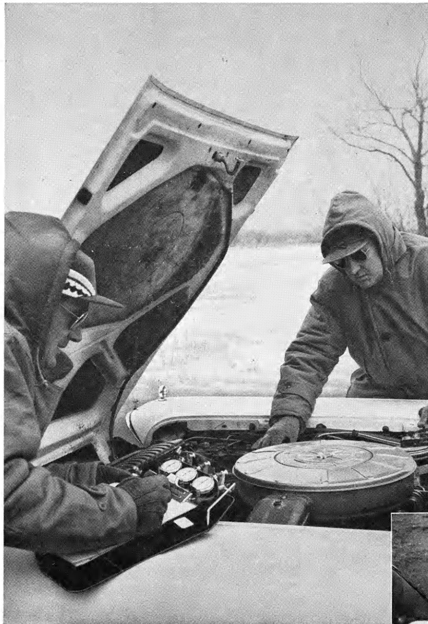
Charles Domke (right) is one of the few men we know who takes a positive delight in having his engine stall in sub-zero weather. He and Mechanic Verland Stout change gasoline blends frequently. When the engine stalls, they try another blend. Their objective, of course, is to find the perfect gasoline under various climatic and road conditions—and the true test is on the road itself!
