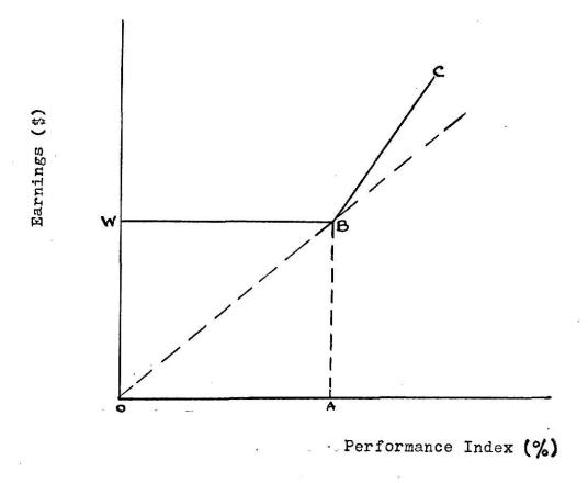
Fig. 4.1 Relationship between the earnings and performance index under the proposed incentive scheme.
