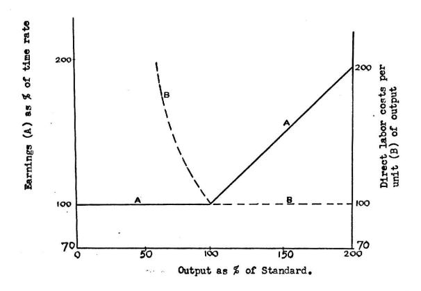
Figure 3.1 Straight piece-work system.
