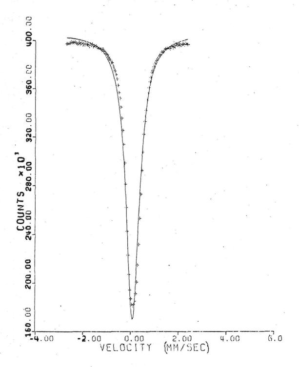
Figure VIII. Source - <sup>57</sup>Co(Pd); Absorber - annealed foil.
