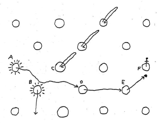
the line containing them both, the pair will be stable and will not spontaneously anneal. The number of such pairs produced increases with the energy of the primary knock-on; at 100 eV, at least one pair will be produced, while at 400 eV as many as eleven pairs may be produced (depending on the initial energy). In the 1965 paper, the authors found that the number of Frenkel pairs produced at energies up to 1500 eV approximately follows the relation:
