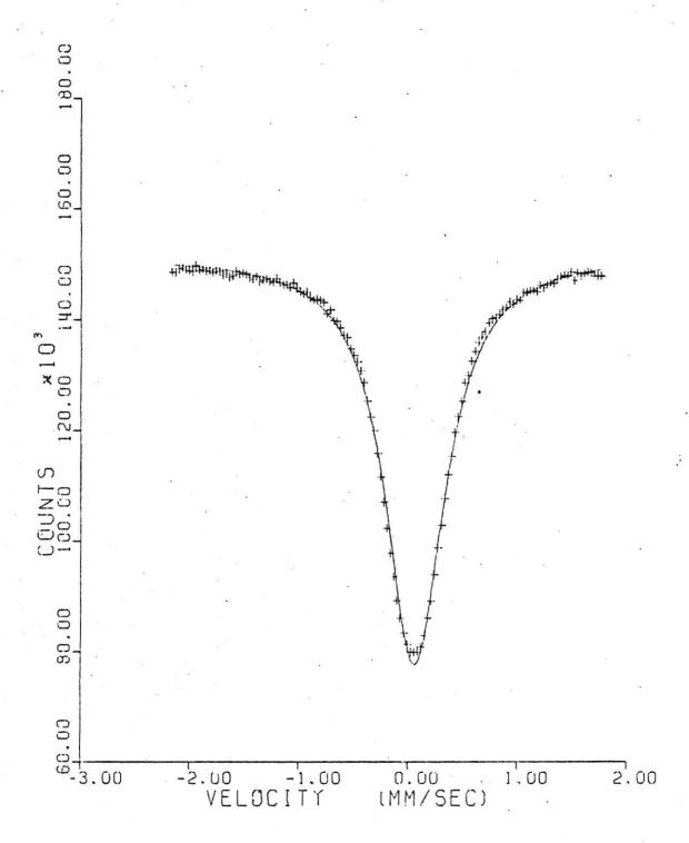
calibration for the spectrum collected during irradiation was made with a  $^{57}\mathrm{Co}(\mathrm{Pd})$  source.
