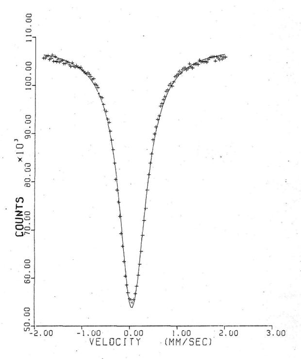
Figure X. Source - <sup>57</sup>Co(Pd); Absorber - ferrocyanide.
