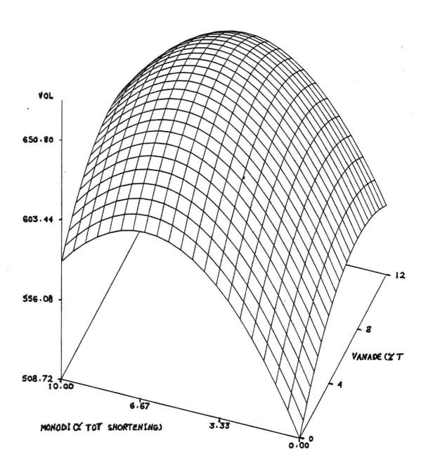
Fig. 18. Three-dimensional response surface of cake volume (cc) for straight grade flour (MMD = 17  $\mu$ , twice reduced) as a function of Monodi and Vanade.
