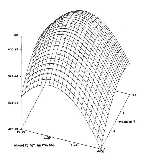
Fig. 17. Three-dimensional response surface of cake volume (cc) for straight grade flour (MMD = 19  $\mu$ , once reduced) as a function of Monodi and Vanade.
