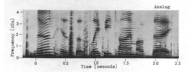
Figure 5. Spectrogram of the sentence "Noon is the sleepy time of day." spoken by a normal hearing speaker.
